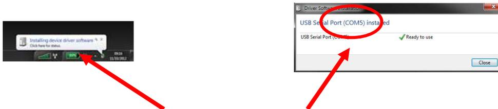
Once USB cable plugged, this popup window indicates that installation has started. By clicking on it you will be able to monitor its progress and, at the end, to know the COM port number associated to the cable (COM5 in this example). This com port number will have to be specified in DATAVIEW config-set in order to be able to use the USB cable to connect to  $\mu$ -BOX and J-BOX.
